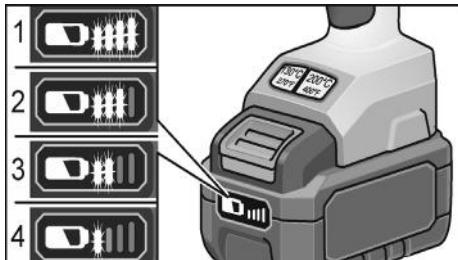
The indicator goes out after 5 seconds. If one of the LEDs flashes, the battery must be recharged. If none of the LEDs light up after the button is pressed, the battery is faulty and must be replaced.
