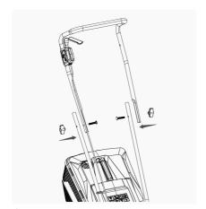
Note: Make sure the wing nuts (5) and mounting bolts (5-a) are properly tightened before using the product.
